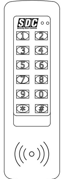
The *EntryCheck™* 923P Indoor/Outdoor Keypad is a surface mount digital keyless entry system designed for access control applications. The backlit keys are bright and, easy-to-read. A heavy cast vandal resistant housing design with mounting plate allows the 923P to be mounted on a rugged surface or on a standard single-gang electrical box.
